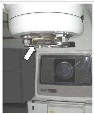
Figure 2 Box fixed at the head of the LINAC (see arrow).
