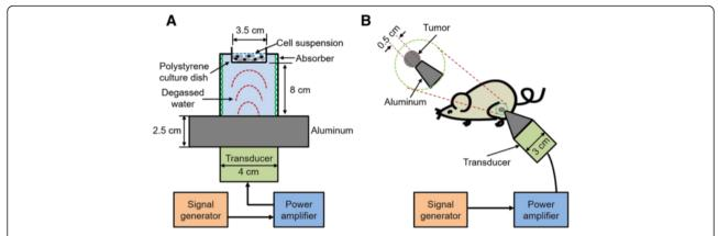
Fig. 1 Schematic diagram of low-intensity ultrasound device and the experimental setup. The tone-burst ultrasonic transducer (1.1 MHz center frequency, 10 % duty factor, 100 Hz pulse repetition rate) for the in vitro (a) and in vivo (b) experiments
